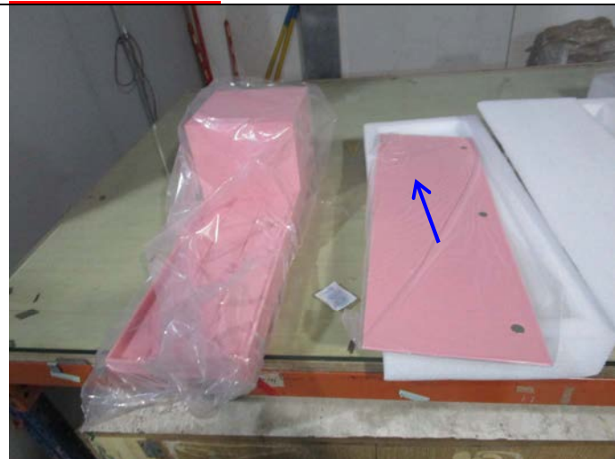
The showcase backplane is incorrectly used and lacks a magnet
